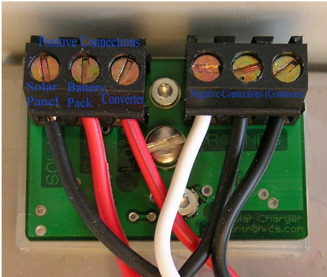
The terminal blocks on the Solar Charger circuit provide connections for the battery pack, the solar panel, and then to the battery converter. Note that each of the three screws on the right side are connected together, and are the 'ground' connections. Each of the
